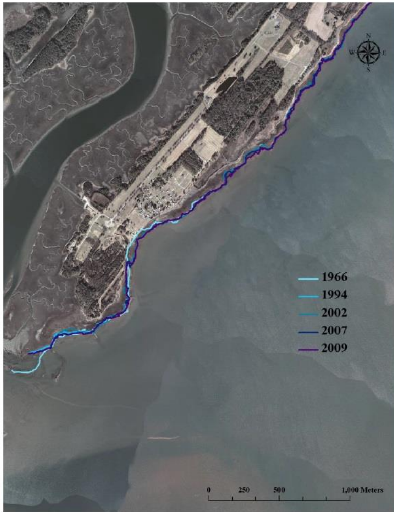
Figure 58: Upshur Neck shorelines and rates of erosion.
